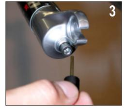
4. With a 5 mm hex wrench, loosen the shaft bolts five turns and firmly tap them with a plastic faced mallet to separate the shafts from the lower tubes.
