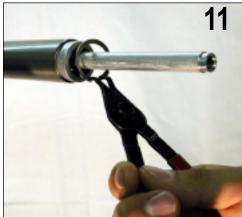
12. Carefully remove the base plate assembly from the U-Turn plunger shaft. Replace the assembly as necessary.
