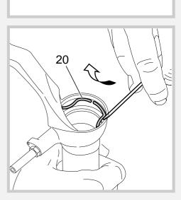
Fit the slider protector **(A)** onto the slider and remove the oil seal **(21)** with the help of a large screwdriver.
