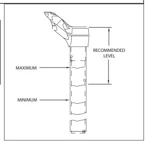
level is different for each model See Figure 7. It is recommended that you replace your oil at least once during the year, twice if it has been contaminated with dirt, mud, or other foreign substance. Use SAE 5WT Maxima fork oil or equivalent.
