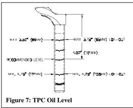
To check the oil level: remove only the compression damping assembly located in
