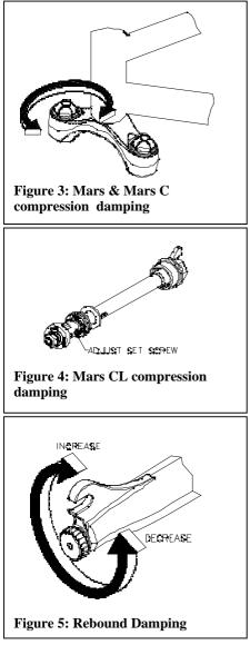
MCU's that better fit your weight and riding style, having the air pressure set mid to low range, and increase the rebound damping to eliminate "top out".
