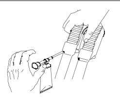
**Figure 6: Lubricating The Bushings**
